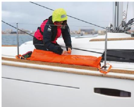
*The Walden system is only secured to the boat's handrail once there is an emergency; no preparation is needed before putting to sea*
