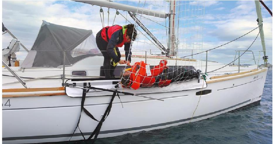
*Assembly is simple: a webbing strap is used to fasten the device to the railing stanchions. It should be unfolded once in port in order to adjust the immersion depth of the net.*
